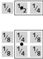
Figure 6 Cosited filters for subsampling use weights that cause the computed chroma sample to be located exactly on the site of a luma sample.
